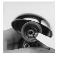
6. Thread the extraction tool into the back of the piston.
