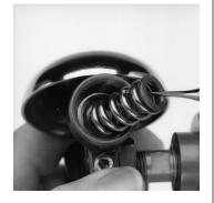
4. Use retaining-ring pliers to remove the retaining ring. Discard the retaining ring.
