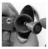
Using retaining-ring pliers, install a new retaining ring. Insert the ring with its flat side facing you. The ring must seat in the groove located about 1/16" above the piston.
