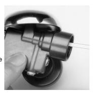
4. Using the O-ring removal tool remove the piston O-ring and the piston plug O-ring. Discard these o-rings.
