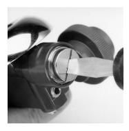
Verify proper Audi-Larm operation by performing the required ring-up, set-point, and ring-down tests specified in the Audi-Larm Audible Alarm Tester Instructions. **Note:** Upon completion of Audi-Larm assembly test procedures, perform the following step.
