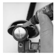
14. Ensure cylinder valve is fully closed. Open the bypass valve to release air pressure, then remove the Audi-Larm Assembly from the Alarm Tester. When you have completed the Audi-Larm Assembly repair and adjustment procedure, check the alarm for air leaks. Refer to the Audi-Larm Leak-Testing section.
