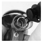
5. Unscrew and remove the piston plug, and the O-ring.
